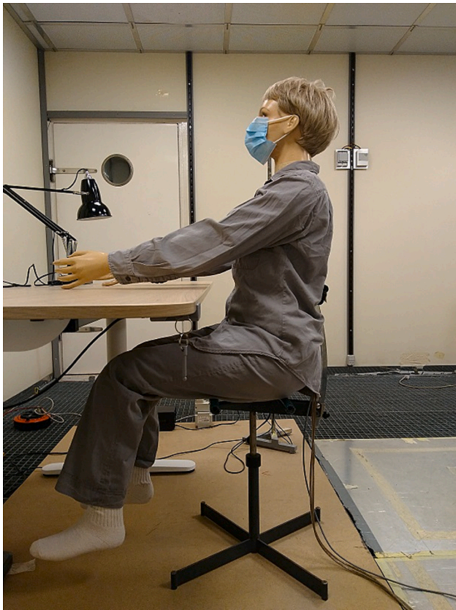
Fig. 2. Thermal manikin dressed in standard clothes, seated in the reference chair (Chair #1) and wearing a surgical facemask.
